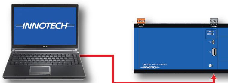
Figure 4-5: Connection from Laptop to OMWEB02 via Ethernet
