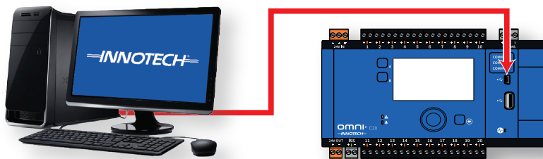
Figure 4-1: Connection from Computer to Omni via USB Mini-B
