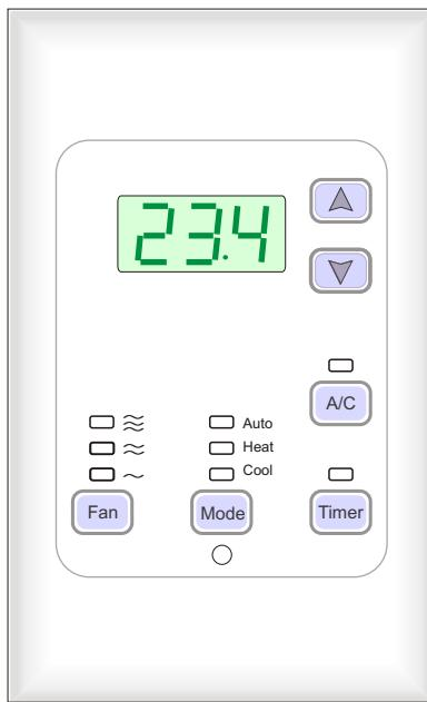
The **A/C** button will switch the unit on or off. The display shows the sensed temperature until either of the **▲** or **▼** buttons are depressed. The set point will be displayed and continuing to press either the **▲** or **▼** buttons will increase or decrease the set point. If the **▲** or **▼** buttons have not been depressed for 5 seconds the display will revert to the sensed temperature.
