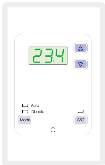
The **A/C** button will switch the unit on or off. The display shows the sensed temperature until either of the **▲** or **▼** buttons are depressed. The set point will be displayed and continuing to press either the **▲** or **▼** buttons will increase or decrease the set point. If the **▲** or **▼** buttons have not been depressed for 5 seconds the display will revert to the sensed temperature.
