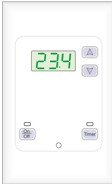
The button will switch the unit on or off. The display shows the sensed temperature until either of the or buttons are depressed. The set point will be displayed and continuing to press either the or buttons will increase or decrease the set point. If the or buttons have not been depressed for 5 seconds the display will revert to the sensed temperature.
