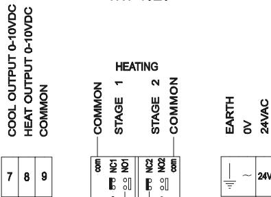
\* Note : Terminal 9 and Earth are Internally Connected.
