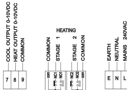
\* Note : Terminal 9 and Earth are Internally Connected.
