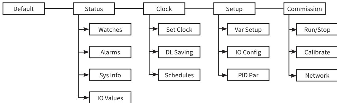
The display has up to 5 programmable watch pages, each with its own user defined description. Each page displays 5 points of information and allows access to the status of all I/O values and system information. The user can set clock/schedules variables and calibrate inputs. All information is displayed in English with standard engineering units.
