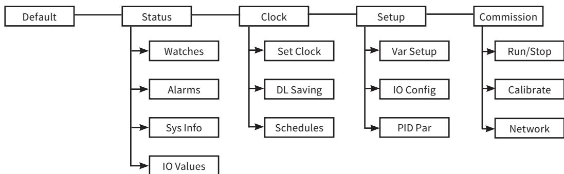
The display has up to 8 programmable watch pages, each with its own user defined description. Each page displays 10 points of information and allows access to the status of all I/O values and system information. The user can set clock/schedule variables and calibrate inputs. All information is displayed in English with standard engineering units.
