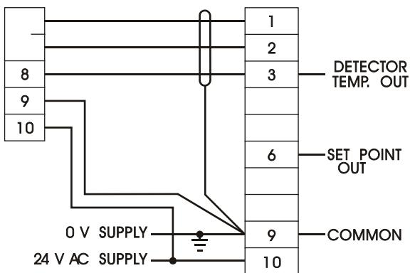
Screened cable should be used to reduce EMI.
