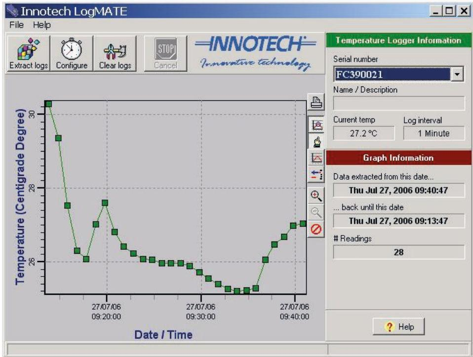
If a temperature logger is connected to the computer USB port, the graphical application will automatically detect its presence and display and continuously update the information shown in the "Data Logger Information" section of the screen.
