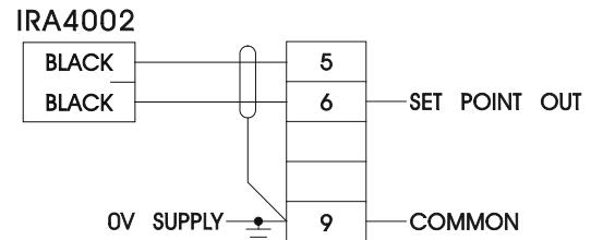
Screened Cable should be used to reduce EMI.
