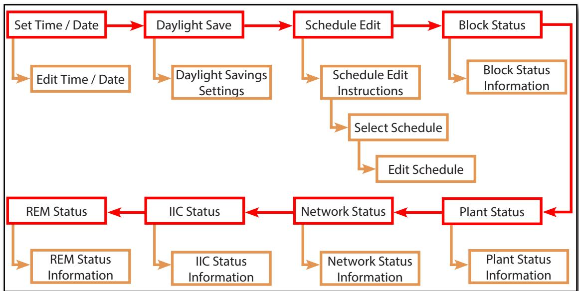
The HMI provides access to various system variables and parameters. It supports 8 function pages, each with 32 points of data such as status and set points. Each function page can be configured with user specific information, and labelled for easy identification using the inserts on the Genesis II cover. Access to the HMI is controlled with multilevel password protection. All information is displayed in English with standard engineering units.
