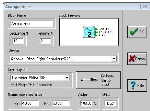
**Gen2Config** contains a wide variety of control functions, ranging from the simple digital logic functions of AND, OR and NOT to more complex blocks such as a scheduler, timer or humidity calculation. In all, the 40 blocks available can be combined in countless ways to produce configurations tailored precisely to your needs.
