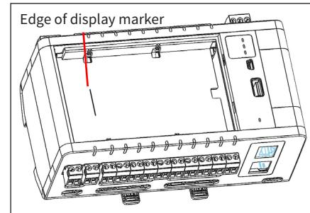
Display plate removed from controller.
