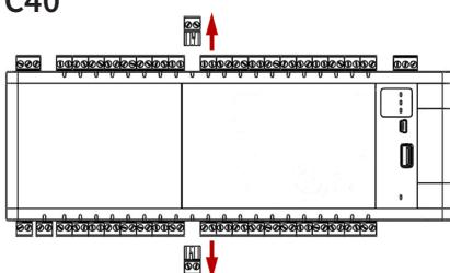
Remove UIO terminals **9** and **29** from the C40 Controller to reveal the snap hook release port.
