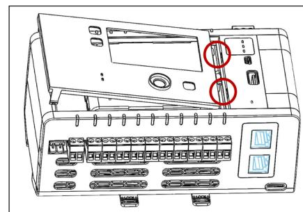
Insert the Faceplate for the OMH01. Start by inserting the tabs on the right side into the corresponding slots on the Omni.
