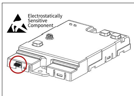
Remove the display from the packaging and foam from the pins. When handling the remote display unit it is very important to treat the exposed connector pins with care. **Avoid handling the pins at all.** They are sensitive to both physical abuse and electrostatic discharge.
