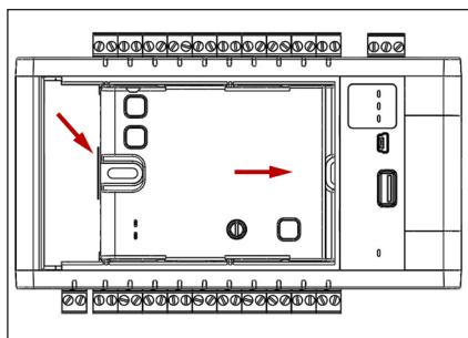
If you experience any significant resistance, stop and try again, the pins may not have perfectly aligned - **DO NOT FORCE**. The OMH01 is "home" when the display is aligned with the edge of display marker in the display bay shown in step 4.
