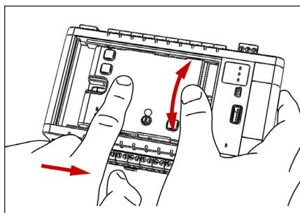
Gently push the OMH01 to the right with your left finger on top of the display. Using your right thumb wiggle the display up and down to seat the pins. Then a final light push from the left is required to "click lock" the OMH01 into position.
