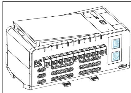
Both sides of the Faceplate should now have popped above the surface and the Faceplate can be lifted off (The C14 may need some assisted levering from the face of Omni to achieve this).
