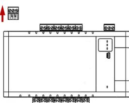
Remove the **24V IN** terminal from a C14 Controller to reveal the snap hook release port. (There is only one on the C14)
