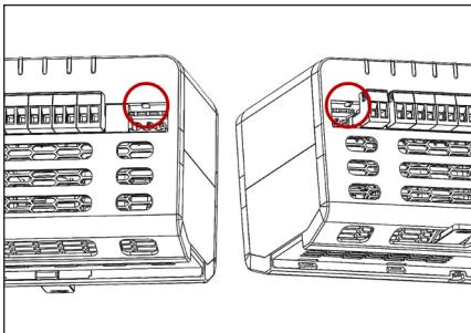
Locate the Snap Hook Release Ports where the plug in terminals were removed.
