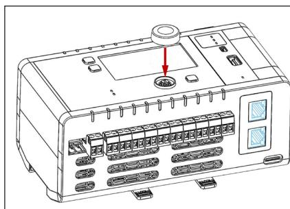
Place the Dial onto the shaft and press home.
