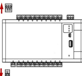
Remove the **24V IN**, and **24V OUT** terminals from the C20 Controller to reveal the snap hook release port.
