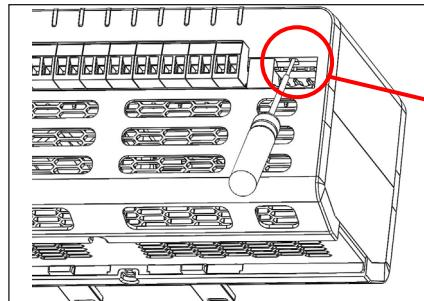
Insert a small flat bladed screwdriver into the hole on an angle, pointing toward the front face of the controller.
