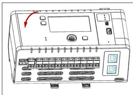
The Faceplate for the OMH01 can then be pressed flat into the Display Bay opening.
