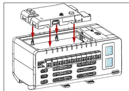
Place the OMH01 unit into the Display Bay of the Omni enclosure. **Ensure the enclosure guide pins align** with the slots on the OMH01. The display will be slid into place in step 9.
