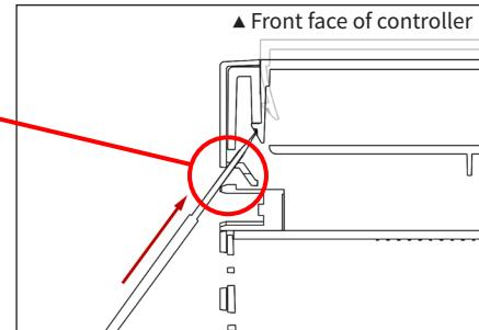
The screwdriver should be able to engage with the Snap Hook, and with a light **pressing** action be released. **Push the screwdriver forward, do not use a lever action.** The corner of the Faceplate should be sitting above the Omni's Face.
