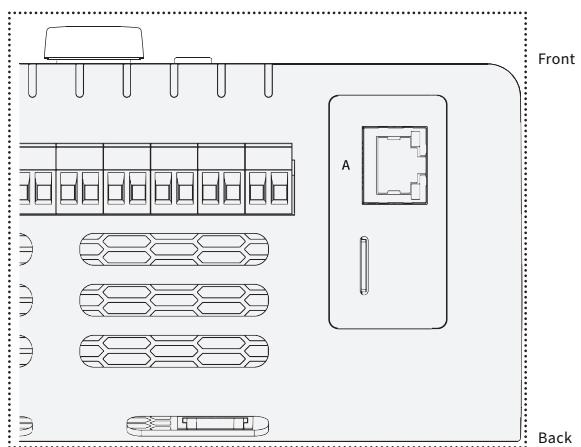
**!** When mounted on DIN rail, the Ethernet RJ45 port(s) and MicroSD slot are located on the **bottom** of the controller.
