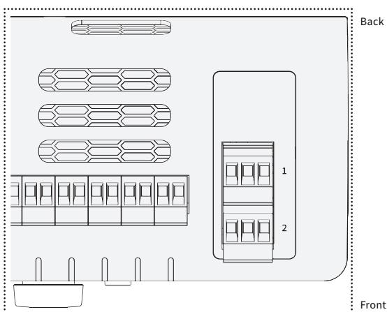
**!** When mounted on DIN rail, the RS-485 Comms port(s) are located on the **top** of the controller.
