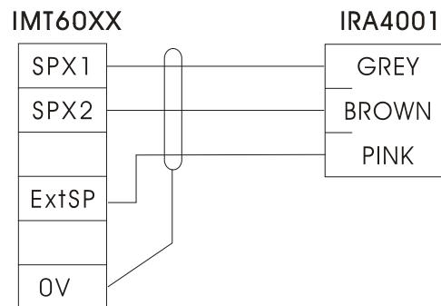
Screened Cable should be used to reduce EMI.
