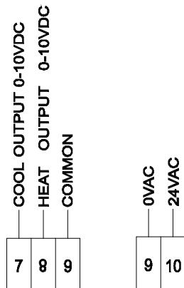
*\*\* Note : Terminal 9 and Earth internally connected. \*\**
